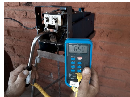
Pyrometer indicating proper blade temperature of 650°C.
